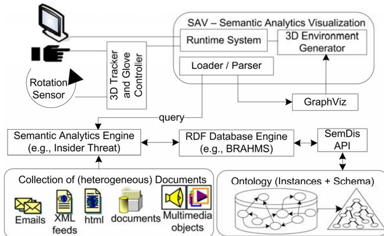
Fig. 2. System architecture of SAV.
