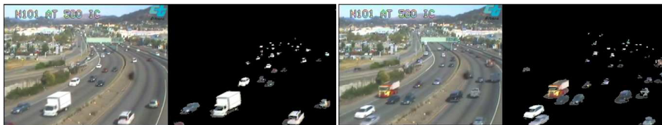
Figure 3: Performance of SILK on a road traffic sequence (moving car detection) task, with a jittery camera. Two random frames and the performance of SILK on those frames are depicted.
